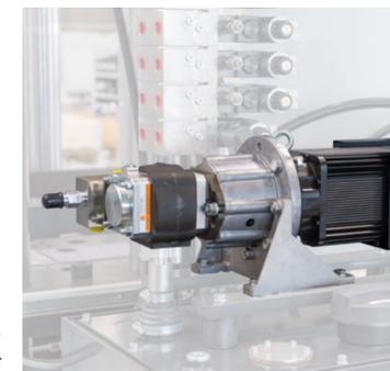
With the intelligent servo-hydraulic MAP.cooldrive drive system, the motor speed adjusts automatically to the actual power requirements during the production cycle.
